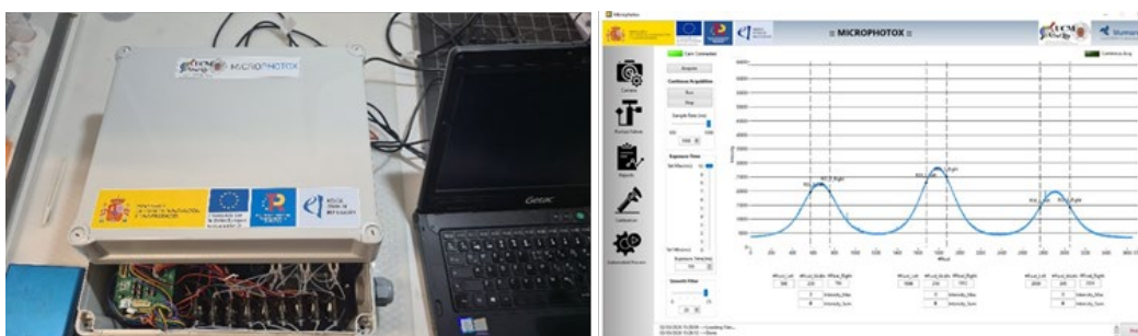
Figure 1. Photograph of the automatic prototype and a screenshot of the dedicated signal control and analysis software developed to simultaneously determine up to 3 mycotoxins in liquid foods.
